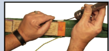
FIBER OPTIC-No Light Transfer (Sling fails inspection)
