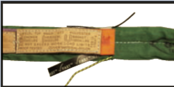
✓CHECK-FAST® EWI PRESENT (Sling passes inspection)
