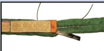
✓CHECK-FAST® EWI MISSING (Sling fails inspection)
