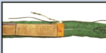
TATTLE TAIL MISSING (Sling fails inspection)
