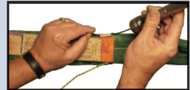
FIBER OPTIC-Transfers Light (Sling passes inspection)
